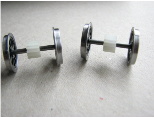
Wheels and gears ready for installation.
