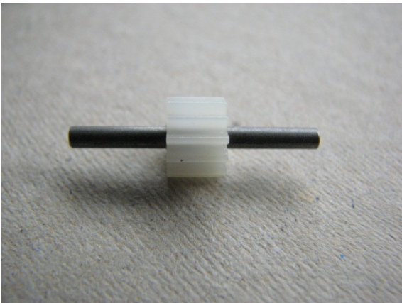
One axle with gear pressed on
